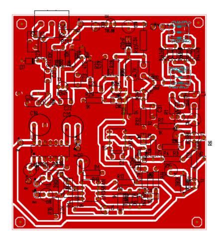
\*Errata: 470 Ohms Resistor is missing in the PCB layout. Add a 470 Ohms Resistor in series with L4. Follow the Schematic.
