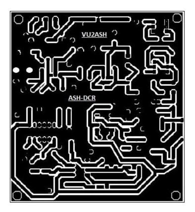
\*Errata: 470 Ohms Resistor is missing in the PCB layout. Add a 470 Ohms Resistor in series with L4. Follow the Schematic and component Side layout.
